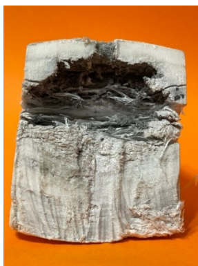
Figure 1. a) Cross section in Endumax XF33 135-layer plate, after being hit with a projectile 7.62x51 mm, v 0 =833 m/s, BFD=28 mm; b) ranges for involved parameters: V 0 – impact velocity, BFD – backface deformation
