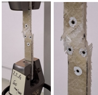
Figure 1. Sample with 8 layers of biaxial prepreg, tested in traction at 500 mm/min
